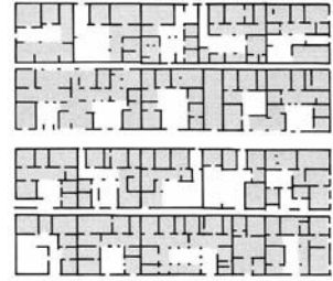
Olynthus, Ancient Greece: Typical 10-house-block layout, each house centered by a south-facing courtyard. (Based on a drawing by J. Walter Graham from plans by Donald N. Wilber in Excavations at Olynthus: the Hellenic House by David M. Robinson and J. Walter Graham.)
